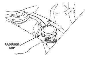
Pressure test the radiator cap. It must hold specified pressure for at least six seconds.
