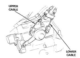
Remove the shift arm bolt and collar.
