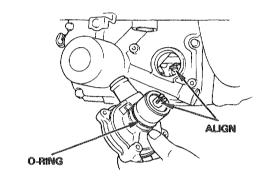
Install a new O-ring onto the pump cover.
