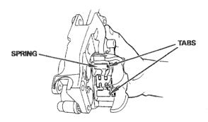
Install the new pads in the caliper.
