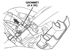
Remove the retaining screws and move the turn signal cancel control unit enough to disconnect the unit connector.
