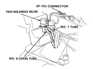
Connect a vacuum pump as shown.
