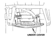
Unfasten the T-stud clips at the lower side of the ignition switch.
