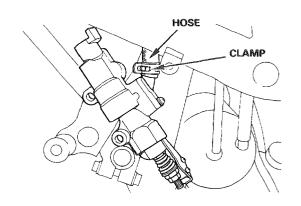
Connect the metal brake line for the front caliper at the rear master cylinder with its nut.
