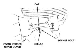
Remove two socket bolts, two flange bolts, and the collars.
