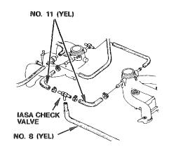
Connect a vacuum pump as shown.
