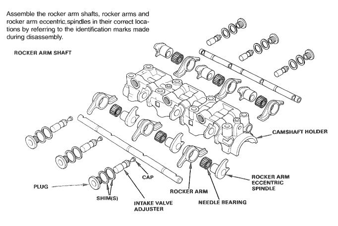
Clean the camshaft holder thoroughly. Blow through all holes and passages with compressed air.
