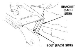
Remove the fairing inner bolt and nut (each side).
