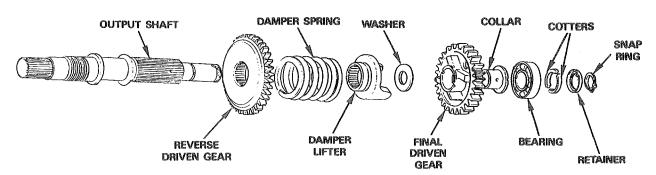
Install the reverse driven gear, damper spring, damper lifter, and washer onto the output shaft.
