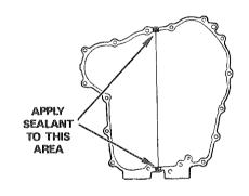
Install a new gasket and dowel pins.
