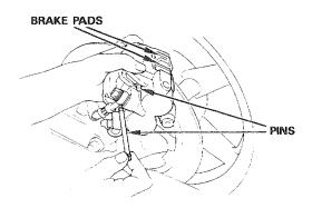
Place the pad pin retainer over the pad pins. Push the retainer down to secure the pins.
