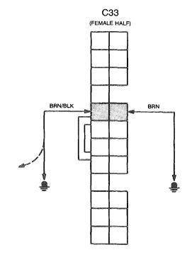
With ignition switch ON, cruise switch ON, engine stop switch in RUN, and ground GRN/BLK wire of the cruise valve relay, remove jumper at BRN circuit while observing throttle. Cruise control actuator releases throttle.
