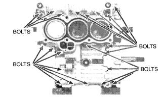
Place the engine with the right crankcase down.
