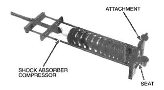
Check the damper for deformation, oil leaking, bending of the rod, or smooth operation.
