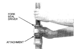
Install the stopper ring and dust seal.
