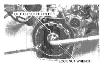
Check the slots in the clutch outer for nicks, cuts, and indentations made by the friction discs.
