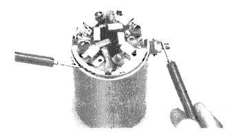
Inspect the commutator bars for discoloration. Bars discolored in pairs indicate grounded armature coils.
