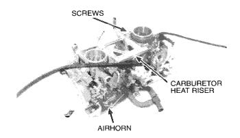
Remove the cotter pin, washers, and collar from the choke linkage sub rod at each carburetor.
