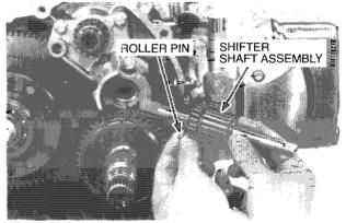
Remove the snap ring and disassemble the shaft assembly.
