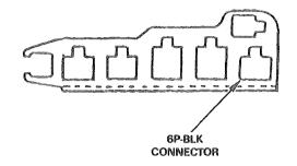
Check for continuity between each terminal as shown below and ground. There should be continuity at each gear position.
