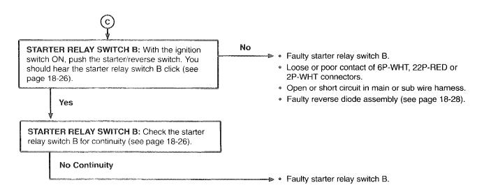
The starter/reverse motor turns in neutral position, but does not turn in gear with the side stand up and the clutch lever pulled in.
