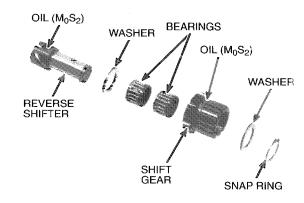
Check the shift gear for rotation.
