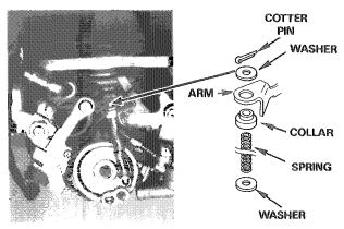
Install the plastic washers, washer, and a new cotter pin on the throttle linkage of the right carburetor.
