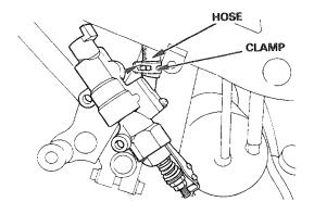
Remove the reservoir bolt, open the reservoir cap, and drain the brake fluid from the master cylinder.
