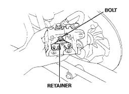
Push the piston all the way in to provide clearance for the new brake pads.
