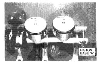
Install piston base "B" (rubber), with its notch toward the connecting rod, under the No. 2 piston (timing belt side).
