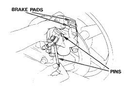
Position the pad spring in the caliper as shown.
