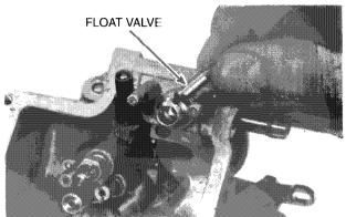
Remove the float valve seat from the carburetor body. Clean the strainer with clean solvent.
