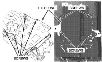
If you want to remove the gauges, remove the rear side of the L.C.D. unit (see above).
