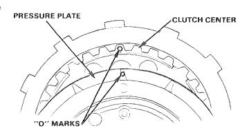
Slide the clutch center assembly into the clutch outer to align the discs and plates.
