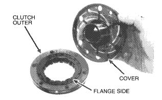
Apply a locking agent to the starter one-way clutch socket bolt threads as shown.
