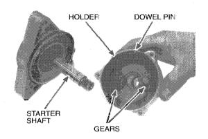
Check the reverse reduction gears for excessive or abnormal wear.
