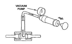
Connect a vacuum pump as shown.
