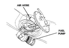
Release the terminal caps from the fuel pump wire terminals.
