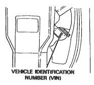
The Vehicle Identification Number (VIN) is located on the right side of the frame near the steering head on the Safety Certification Label.
