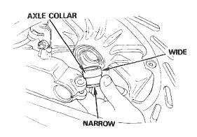
Position the caliper and bracket as an assembly over the disc.
