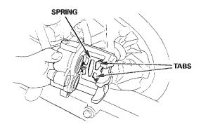
Install the new pads in the caliper.
