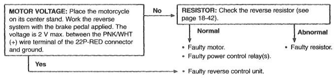
The speed limiter system is not activated at or above 2.5 km/h in reverse.
