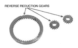
Check the starter reduction gears for excessive or abnormal wear.
