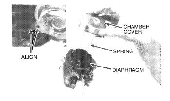
Install the remaining screws of the vacuum chamber cover.
