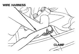
Release the right handlebar switch wire harness from the clamp.
