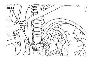
Remove the rear axle pinch bolt and pull the rear axle out of the wheel.
