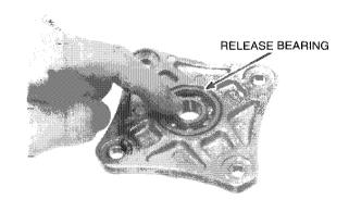
Install the bearing with its mark side facing out.
