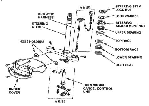
Pack the bearing cavities with grease.
