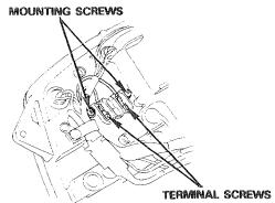
A & SE: Disconnect the 3P-WHT connector to the speed sensor.
