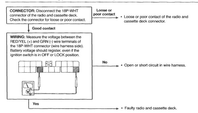
The radio and cassette deck display does not appear on the L.C.D. unit (A and SE models).
