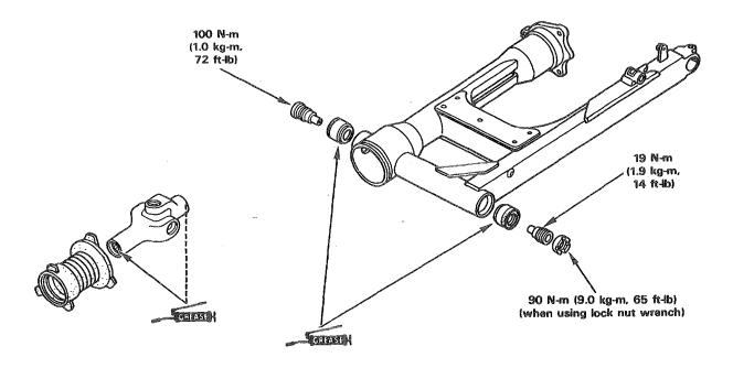
Lubricate the universal joint splines with grease.
