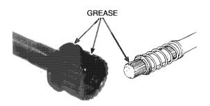
Insert the drive shaft into the pinion joint spline grooves.
