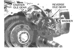
Remove the reverse shifter shaft assembly.
