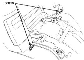
Pull back on the rear section to slide the lower rear frame tubes away from the loosened bolts.
