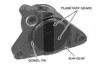
Install the gear holder, aligning the holder groove with the dowel pin.
