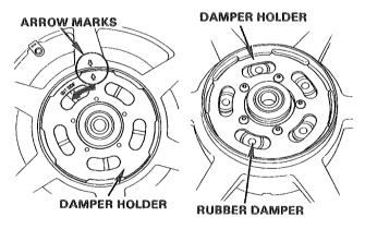
Install the driven flange to the wheel hub.
