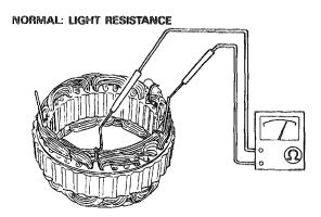
Check for continuity between the wire and stator cord. There should be no continuity.
