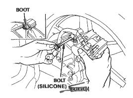
Tighten the caliper bolt, pin bolt, and retainer bolt.
