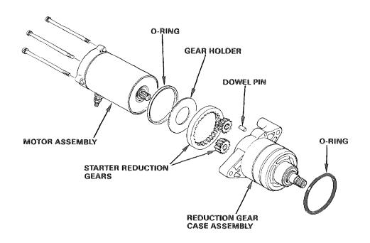
Install the dowel pin into the gear case.
