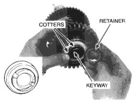
Install the snap ring with the chamfered surface facing the retainer.
