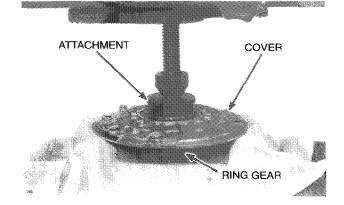
Remove the oil seal from the case cover.
