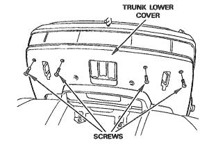
Release the cover grooves from the trunk tabs.
