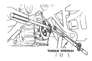
Bend one lock tab of the lock washer up to the lock nut as shown.
