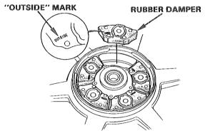
Install the damper holder into the wheel hub.
