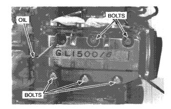
Install the cylinder head rear cover with a new gasket.
