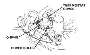
Remove the thermostat from the thermostat housing.
