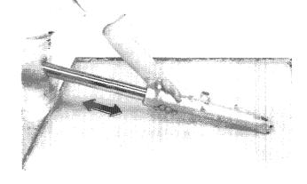
Remove the oil seal, back-up ring, and slider bushing from the fork tube
