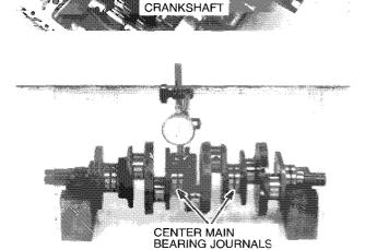
Measure the crankshaft main bearing journals and crankpins with a micrometer for out-of-round and taper.
