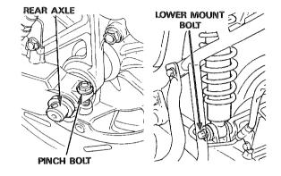
Install and tighten the rear axle nut.
