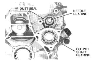
Drive a new output shaft bearing into the cover.
