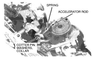
Remove the cotter pin, washer, and plastic washers from the throttle linkage of the right carburetor.
