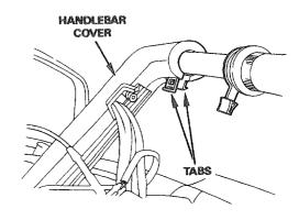
Install and secure the handlebar cover set plates with the screws.
