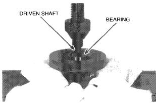
Remove the alternator driven sub gear and gear spring.
