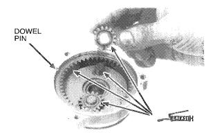
Install the gear holder, aligning the holder groove with the dowel pin.
