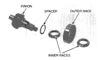
Press the bearing and both inner races onto the pinion gear shaft.
