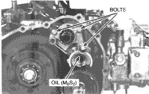
Apply oil to the needle bearings.
