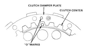
Install the pressure plate, aligning the "O" marks on the pressure plate and clutch center.
