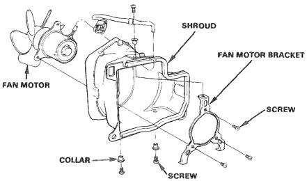
Remove the nut, fan and washer from the fan motor.
