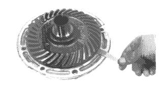
Remove the ring gear, if the clearance exceeds the standard.
