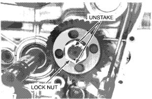
Set the transmission in any gear. Remove the lock nut by turning it clockwise.
