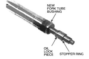
Install the spring seat, spring, and oil lock valve on the piston. Secure them with the stopper ring.
