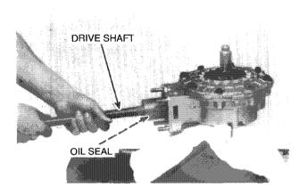
Loosely attach the gear case on the swing arm.
