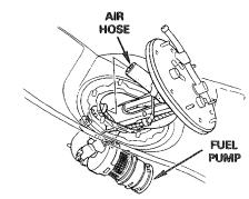
Position the wire clamp over the stud as shown and tighten the nuts securely.
