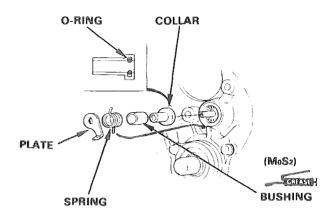
Install the spring, hooking it onto the tab of the output shaft bearing holder as shown.
