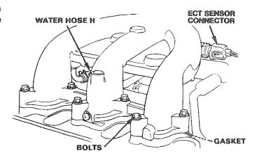
Disconnect the vacuum tube (No. 1, No. 6 GRN) and water hose H from the left intake manifold.
