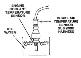
Cool the test engine coolant temperature sensor in the ice water for approximately ten minutes.
