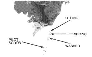
Perform a pilot screw adjustment (see page 4-39) if new pilot screws are installed.
