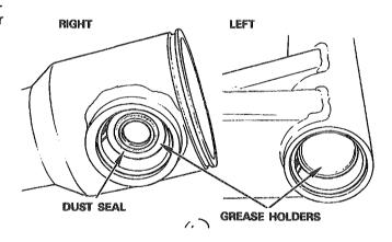
Remove the right outer race with the grease holder.
