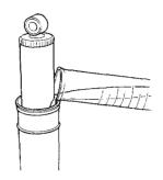
Install the guide bushing in the damper case.
