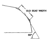
Install a 45 degree finish cutter and cut the seat to the proper width.
