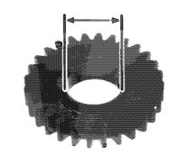
Measure the O.D. of these gear bushings.
