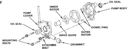
Clean all removed parts thoroughly. Dip them in clean engine oil before reassembly.
