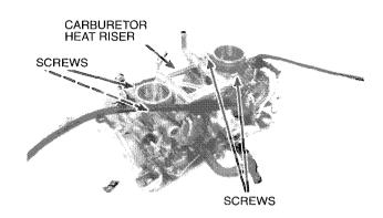
Tighten the carburetor airhorn screws securely. Install new O-rings on the airhorn grooves.
